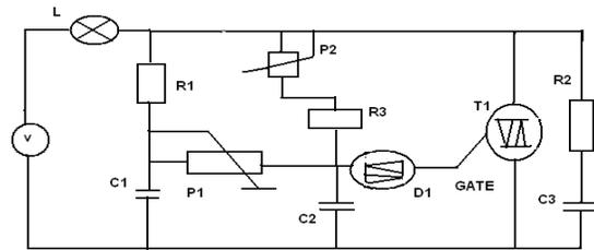
Figure 3: Circuit diagram using TRIAC
