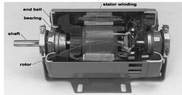
Figure 1: Cross section of Induction Motor
